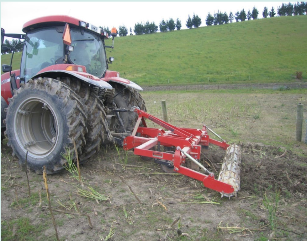
Figure 14: Mechanical soil aeration using a 'Clough pan-aerator' with winged tips for improving soil structure after winter forage crop grazing.
